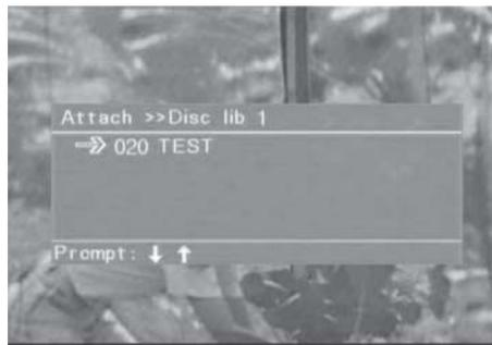
7.3.5 Press up/down button or rotate the knob to move the cursor to the disc name you want to select. You can search the disc with disc name by pressing the [SEARCH] button. (Please refer to "search by disc name")
