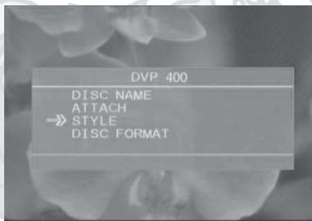
7.4.2 Press up/down or rotate the knob to move the cursor to "STYLE", then press the [ENTER] button to enter the style list. The screen displays as the following picture. The VFD displays style name which the cursor points to.
