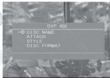
7.2.2 Press up/down button or rotate the knob to move the cursor to "DISC NAME", then press [ENTER] to enter the disc name list, the screen displays the following picture, the VFD displays disc name which the cursor points to.
